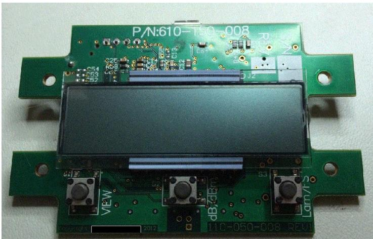
As part of design verification testing, a pre-production unit was tested over a range beyond the spec. Also, power was margined beyond the operating spec. A single electrical issue was discovered involving a diode which had a reverse leakage rating which was higher than it should have been. While it did not affect
